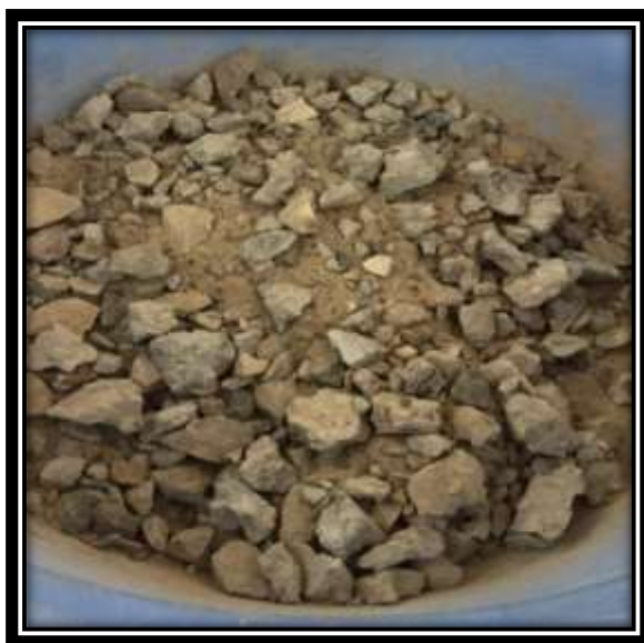
Plate 2. Reclaimed Concrete Aggregate Materials (RCA) Used in This Study
