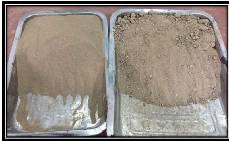
Plate 1. Foundry Sand Used in This Study
